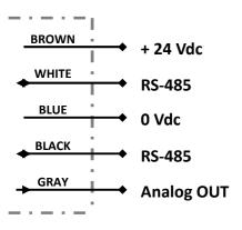
(The type of analogue output can be programmed through the RS-485 Bus)
